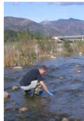
Jason Weiner takes e-coli and fecal coliform grab samples from Sespe Creek.
